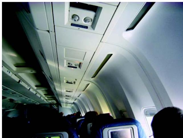
**Figure 1** Economy section in a wide-body passenger aircraft cabin showing several overhead personal service units with their individually controlled gaspers (personal air outlets) and reading lights. The main cabin ventilation supply is provided by sidewall slot diffusers located just below the overhead stowage bins and ceiling slot diffusers located just above the stowage bins near the aisle. IAT photo May 14, 2010.
