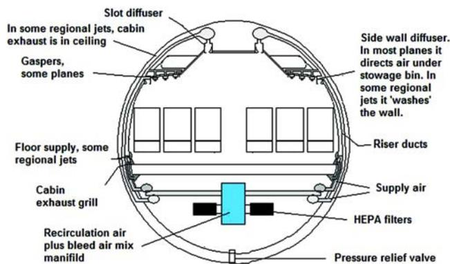
**Figure 1** Aircraft cabin cross section illustrating a cabin environmental control system (ECS) including a cabin ceiling and wall supply and floor exhaust system, as well as some components of a cabin floor to ceiling supply and exhaust system in some regional jets.<sup>25</sup>
