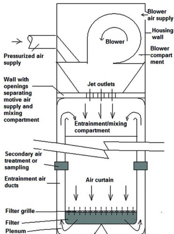
**Figure 11** Air curtain with recirculation entrainment, filtering, sampling (e.g. chemicals for security screening) and possible electronic zapping of flying insects.<sup>25</sup>
