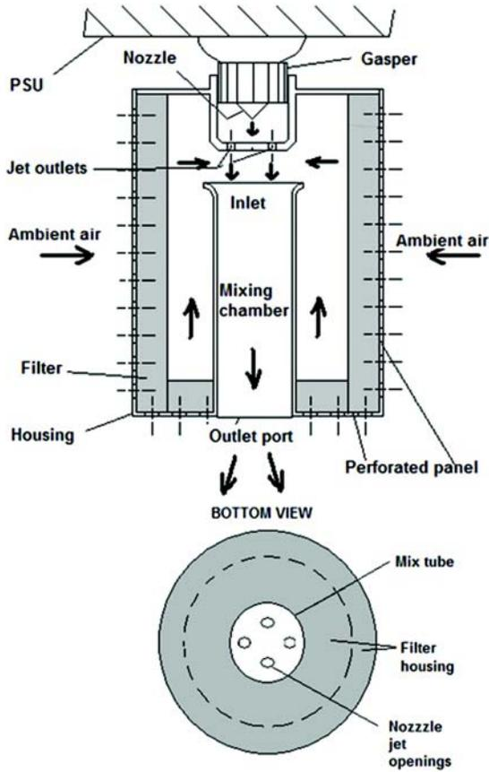
Figure 6 Schematic of a portable Venturi filtered entrainment gasper design.<sup>22</sup>
