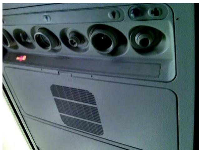
**Figure 2** Personal service unit (PSU) with three gaspers, three reading lights and oxygen masks (not showing) in a narrow body cabin.
