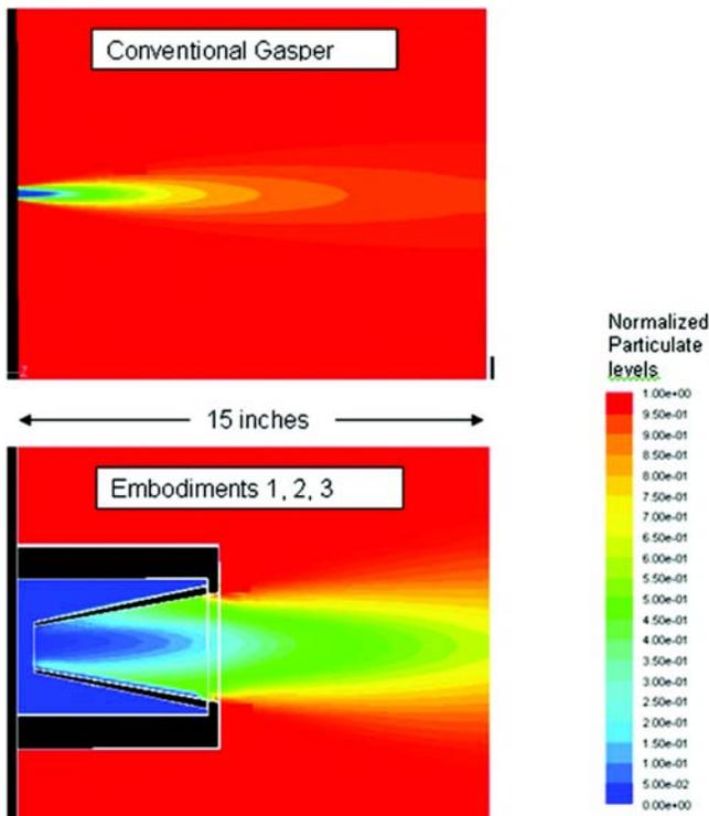
**Figure 4** Mathematical model showing 0.3 micron and larger airborne particulate concentrations with (lower figure) and without (upper figure) filtered entrainment with 60% 0.3 micron filtration. The portable Venturi gasper filtration device can entrain and filter 2.5 times the original 'motive' gasper air supply.<sup>22</sup>
