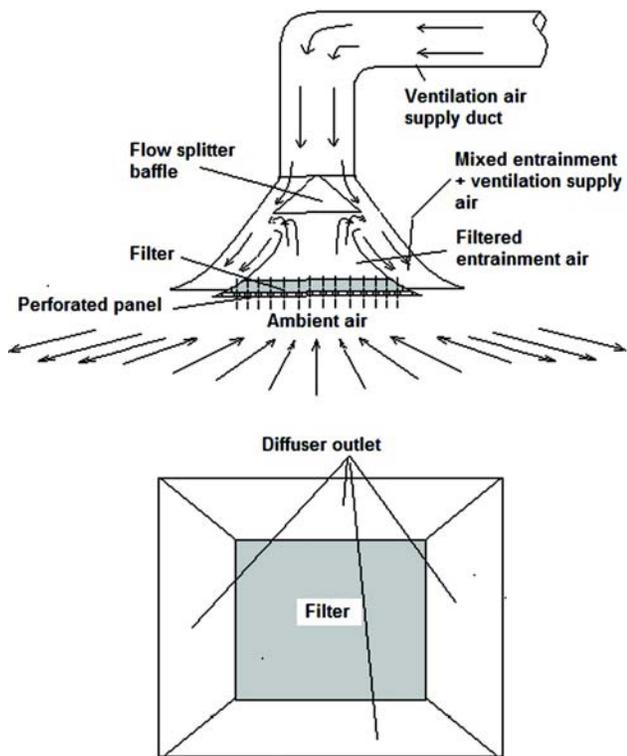
**Figure 10** Example of a square supply air diffuser with Venturi filtration added.<sup>25</sup>
