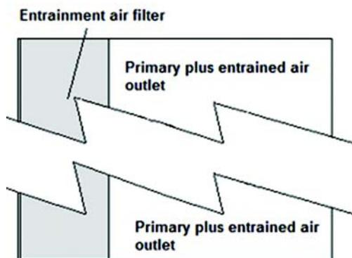
**Figure 8** Slot diffuser with entrainment filtration and/or UV purification on one side the diffuser air outlet. Flow multiplier might be 10 times the motive flow.<sup>25 26</sup>
