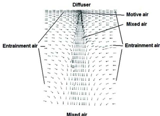
**Figure 3** Mathematical model of the gasper airflow and the lateral entrainment from neighboring areas created. Gasper flow is 3 cfm (1.4 L/s), 95 fps (28 mps) air flow into a cabin at 8000 ft cabin pressure (0.75 atmosphere) illustrating lateral entrainment of air by the motive air flow into a 'motive plus entrainment' mixed airflow in otherwise still air.
