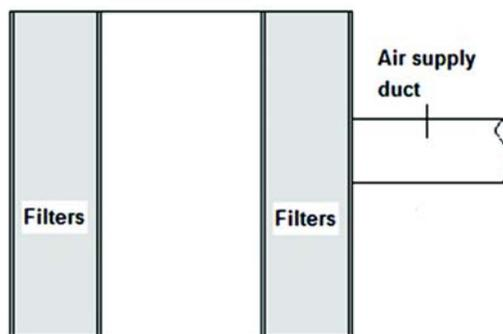
**Figure 9** Slot diffuser with Venturi air filtration and/or UV purification on both sides of the diffuser air outlet. The flow multiplier will be greater with its larger filter area.<sup>25</sup>
