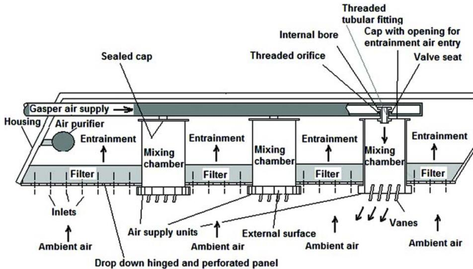
Figure 7 Schematic of a PSU with built-in Venturi filtration. With 60% 0.3 micron filtration entrains 4 times the original 'motive' gasper air supply.<sup>22</sup>
