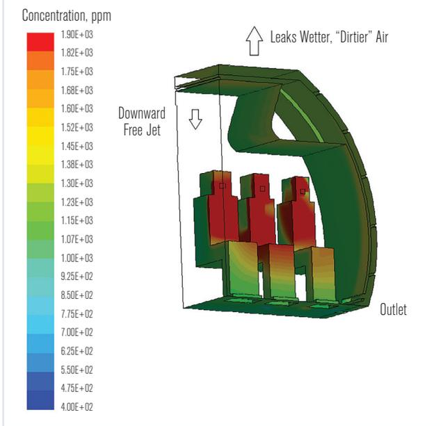
FIGURE 12 Flow pattern for a double aisle cabin with under bin supply nozzle from CFD.
