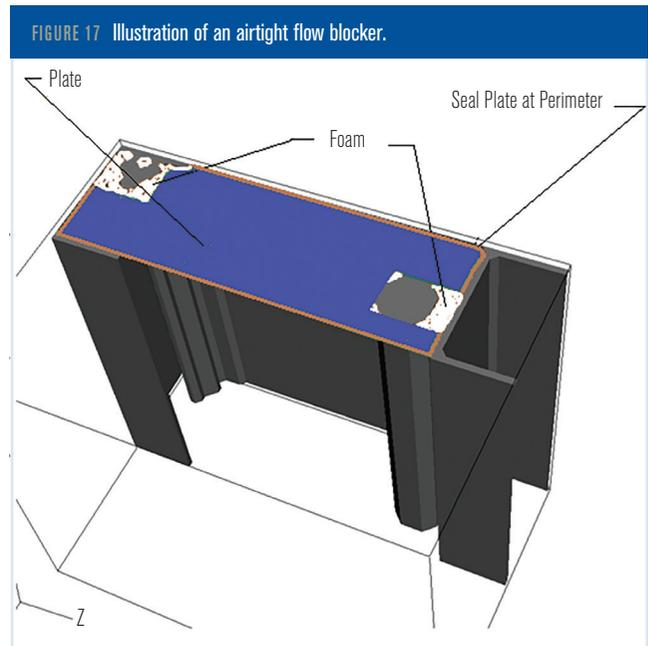
FIGURE 17 Illustration of an airtight flow blocker.
