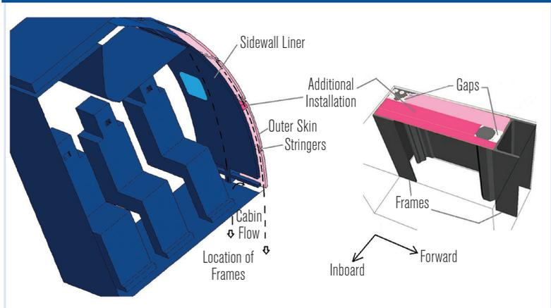
FIGURE 7 A simplified example of bypass ventilation flow loss for basement and airplane cabin.
