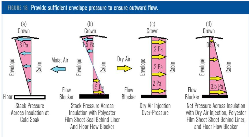
FIGURE 18 Provide sufficient envelope pressure to ensure outward flow.
