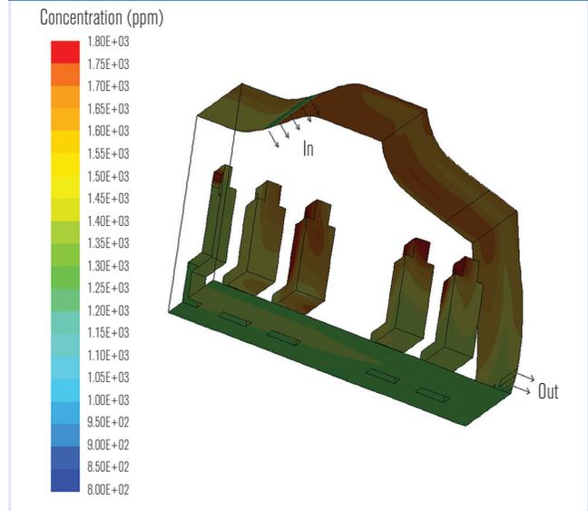
The stack flow through the ceiling panels will divert outdoor air from the cabin and increase the cabin contaminant levels. The ceiling panel is exposed to cleaner, drier air, so condensation would be reduced at the expense of the (reduced) air quality (Figure 13).
