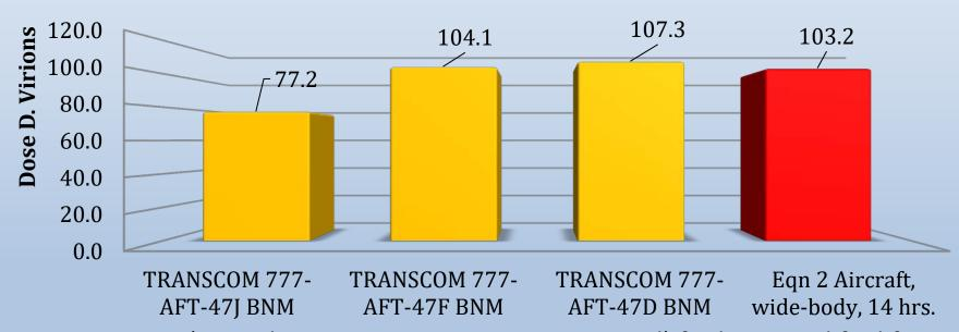
USTRANSCOM (United States Transportation Command) findings modified for the virion shedding rate, virus-free ventilation rate, inhalation rate, occupancy density and exposure times used in Eqn. 1 for the wide body cabin.
